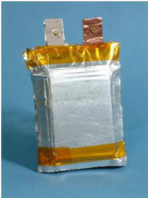
Fig. 1. Photograph of a 7-cell parallel string 175 Ah, 2.5 V module.
