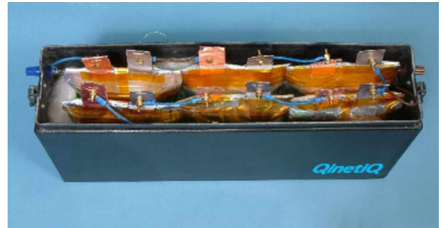
Fig. 2. Photograph showing module connection and configuration.
